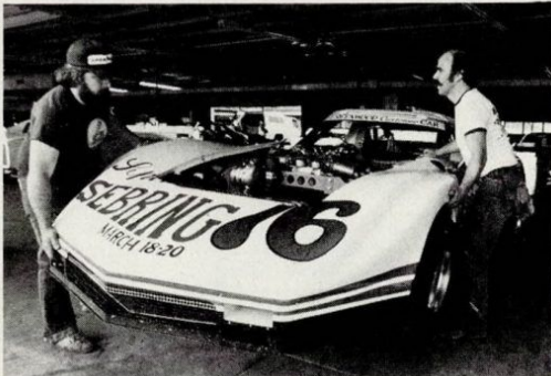
Front fiberglass can be removed and installed without disconnecting radiator as on previous car.
