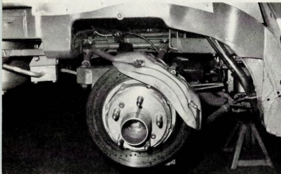
Race car's rear suspension has unequal-length A-arms.
